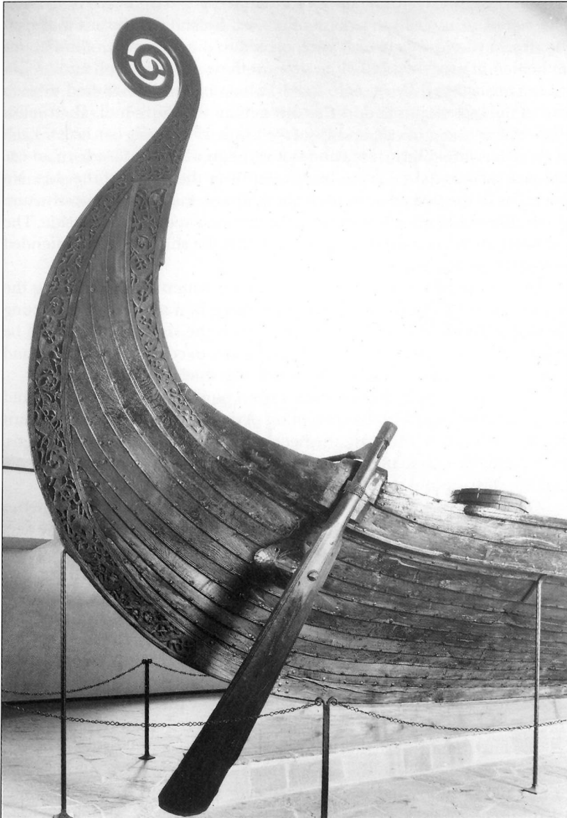
The magnificent stern section of the Oseberg ship showing the deep, blade-shaped rudder. Note the rudder boss and the stout, tapered block of wood reinforcing the gunwale where the rudder neck is secured by means of an adjustable, braided leather band. (University Museum of Cultural Heritage, University of Oslo, Norway)
