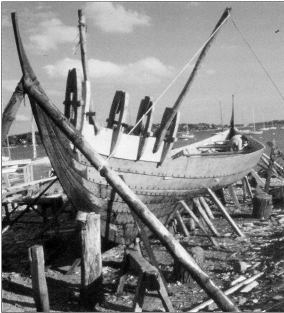
The Skuldelev 3 replica 'Roar Ege' under construction at Roskilde. Note the stocks and the jaw-like clamps that hold the strakes in position. This scene would be familiar to a Norse shipwright 1000 years ago. (Viking Ship Museum, Roskilde)
