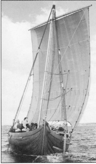
Under her full, woollen sail, the 'Ottar' cruises on Roskilde Fjord. Ample of beam, it is clearly apparent why the sagas refer to these seaworthy vessels as 'swan-breasted'. Ropes employed in the rigging are made from hemp, limebast and horsehair. Note the buntlines running from mast to sail and the sturdy shrouds that support her mast. (Photo Werner Karrasch, The Viking Ship Museum, Roskilde)
