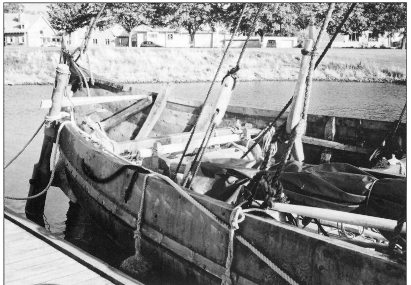
'Ottar's robust construction is clearly evident in this close-up of her stern. Note the tool marks on her hull, the powerful rudder and the windlass that assists in raising the yard and sail. (Author)
