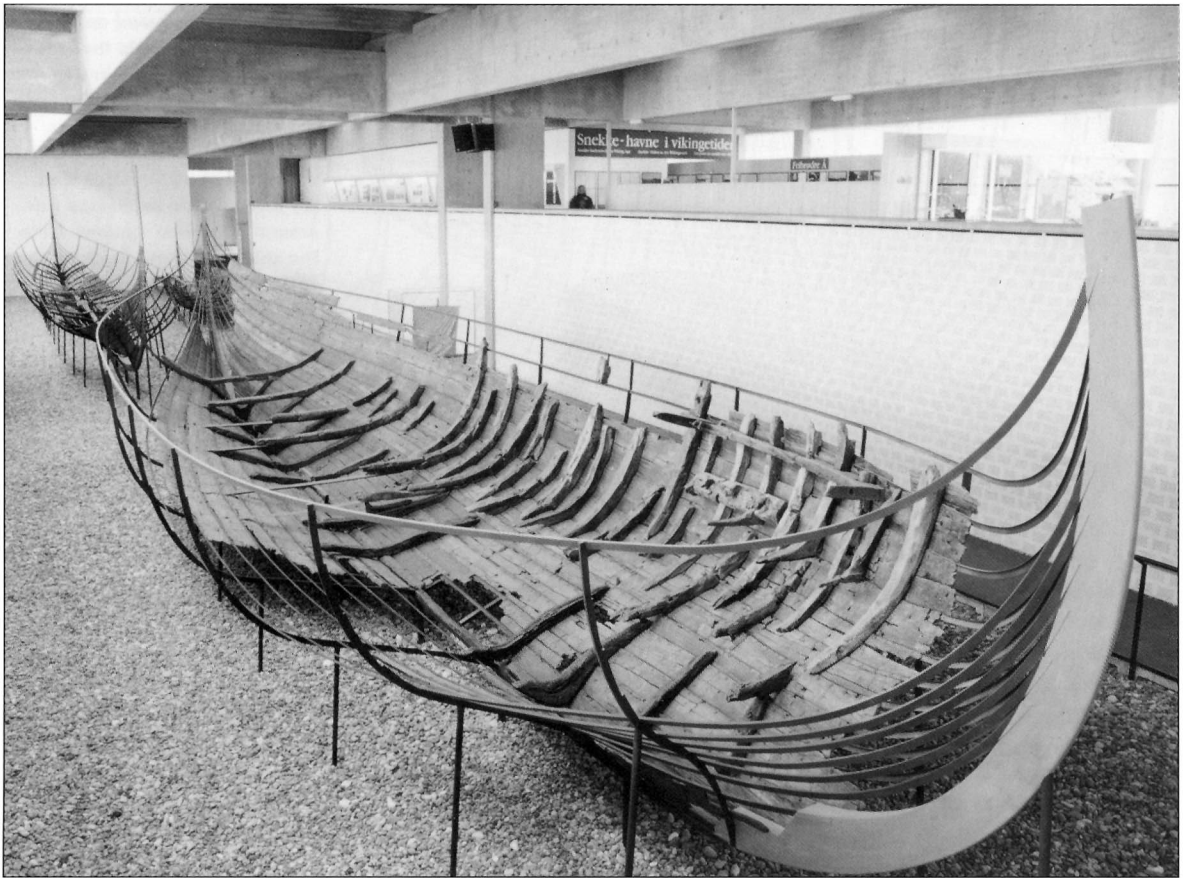
The well-preserved remains of Skuldelev 1. On the forward port side, note the surviving section of the longitudinal stringer rebated into the ribs and below it, the beiti-ass block. (Photo Werner Karrasch, The Viking Ship Museum, Roskilde)
