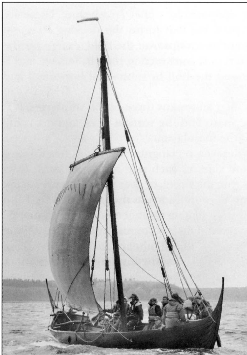
Reconstruction of a large ocean-going knarr , the remains of which were discovered in the harbour at Hedeby/Haithabu. The ship has been estimated at 22.08 metres long, 6.2 metres wide amidships and 2.52 metres high. Note the large hold amidships that would have held in the region of 60 tons of cargo, more than twice as much as Skuldelev 1 . (Drawing: Sune Villum-Nielson, from 'Viking Age Ships and Shipbuilding in Hedeby/Haithabu and Schleswig' (Ole Crumlin-Pedersen 1997)
