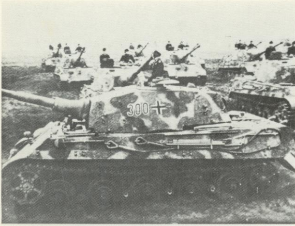
Company of 'Tiger II' ('King Tiger') heavy tanks on manoeuvres. The basic buff-yellow factory scheme was camouflaged at unit level with dark green and brown. These vehicles served in independent heavy tank battalions under direct Army command, rather than as integral units of the individual divisions. (Imperial War Museum)
