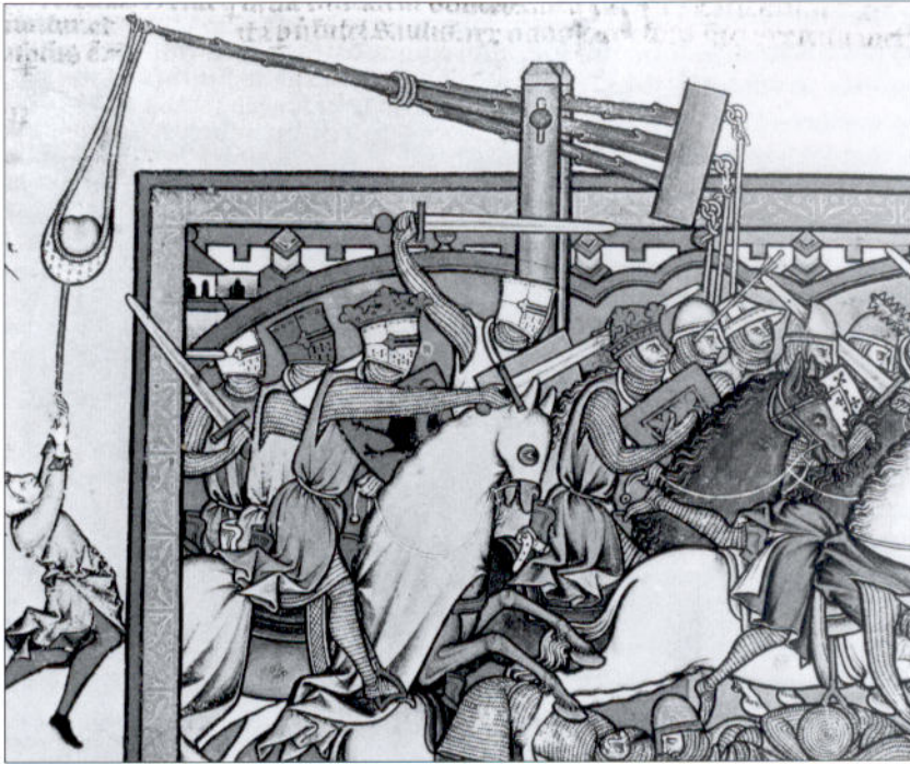
The beam-sling of the man-powered mangonel in this illustration of 'Saul's army destroying Nahash' in the mid-13th-century French Maciejowski Bible is made of roughly trimmed boughs or tree-trunks lashed together with rope. Reinforcing stitches can also be seen in the sling itself. (f. 23v, Pierpont Morgan Library, New York)
