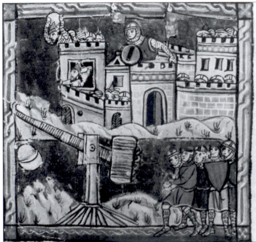
'The Siege of Antioch' in William of Tyre's History of Outremer , made in Acre shortly before the Crusader city fell in the late 13th century. This man-powered mangonel is of a type sometimes interpreted as a half-way form combining both a fixed counterweight and a team of rope-pullers. (Ms. 828, f.33r, Bib. Munic. Lyons)
