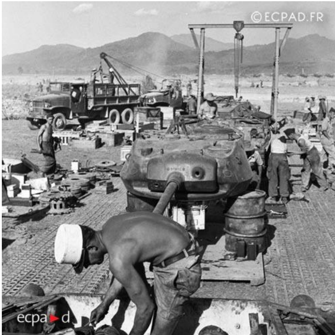
A 2e CREBLE legionnaire at Dien Bien Phu , during M24 Chaffee tank assembly. https://foreignlegion.info/battle-of-dien-bien-phu/
