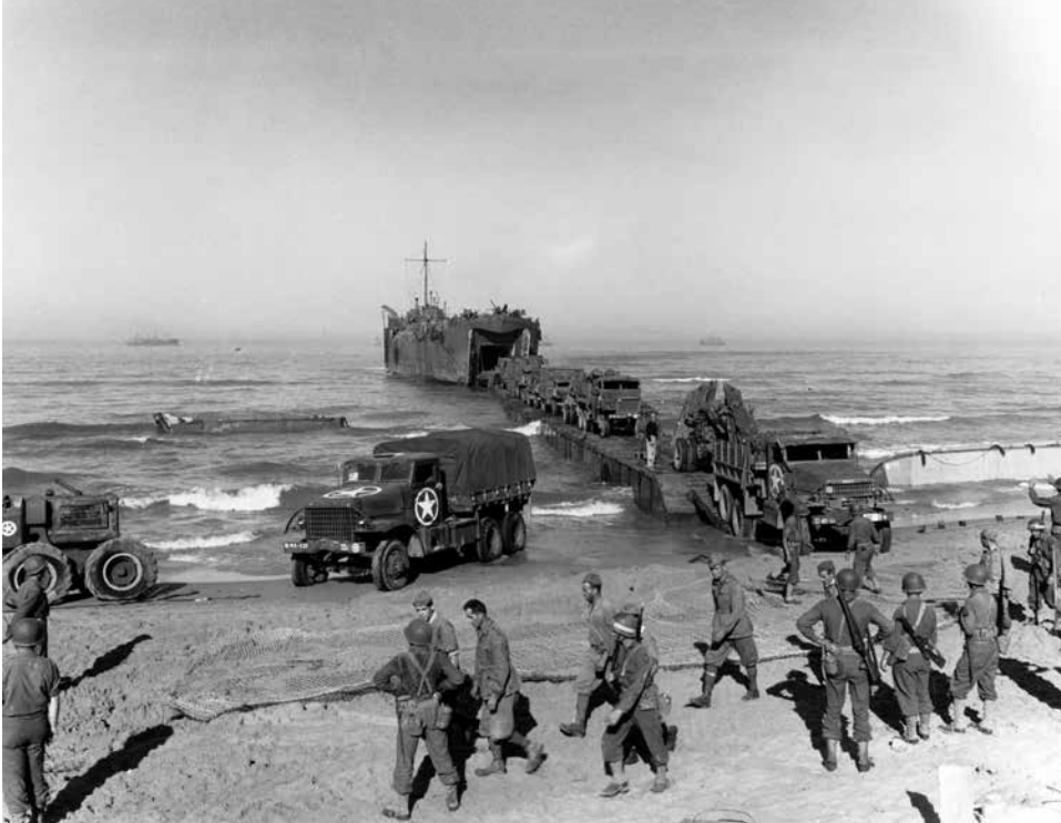
USS LST-336 unloads trucks over a pontoon causeway, near Gela, Sicily, July 1943. (National Archives and Records Administration)
