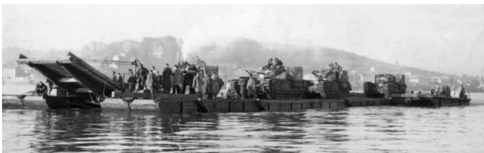
British rhino ferry in original configuration with rhino tug carrying a load of Churchill heavy tanks. (Image provided by Andrew Hussey, Manston, UK)
