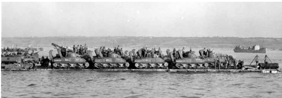
Rhino ferry RHF-18 carrying a load of armored vehicles to Omaha Beach with a freeboard of inches in places. (US Navy Seabee Museum, Port Hueneme, CA)
