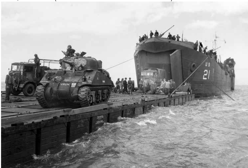
USS LST-21 offloading British armor and vehicles onto a rhino ferry, possibly RHF-100, off Gold Beach, 6 June 1944. (National Archives and Records Administration)
