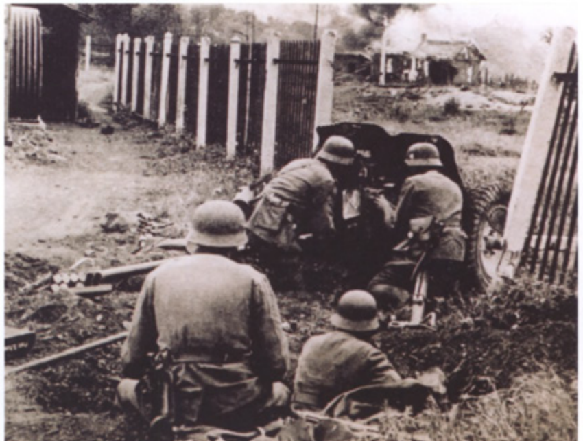
A 37mm Pak 35/36 in action. Developed from 1934 it was one of the most technologically advanced of its time, only to prove dramatically outdated in 1940 against the heavily armoured French and British tanks that it could not penetrate, eventually being nicknamed the 'door knocker' by its crews. (Private collection)
