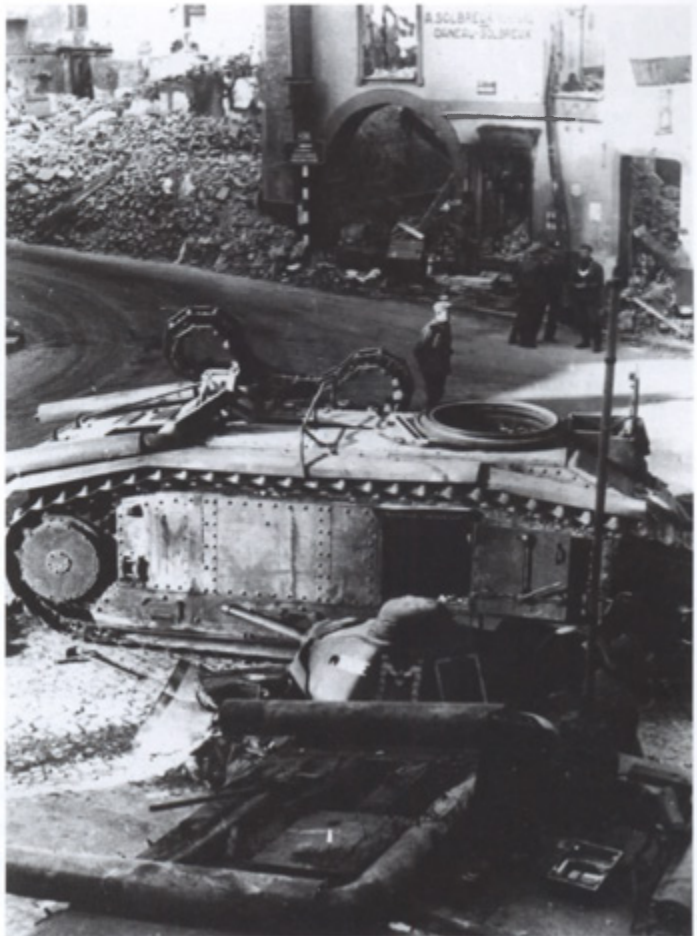
A destroyed French Char B1 bis heavy tank, May 1940. These were used at Stonne to counterattack Guderian's breakthrough at Sedan and proved invulnerable to the standard 37mm anti-tank gun. The Germans destroyed them using either heavy artillery or anti-aircraft guns. (Carlo Pecchi)
