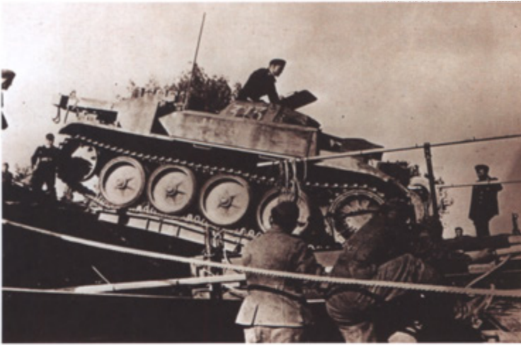
The Panzer II Ausf. L 'Luchs' was the last version of this tank, a reconnaissance vehicle of which only 100 were produced. In the last years of the war the Panzer divisions lacked a suitable fully tracked, armoured reconnaissance vehicle. (Carlo Pecchi)
