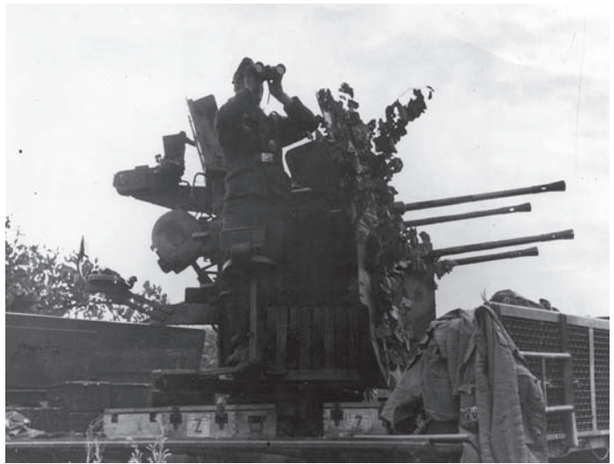
A Luftwaffe 20mm Flakvierling 38 on a self-propelled mount in Normandy, 1944. By this stage anti-aircraft artillery was the main tool available to the Germans to counter the ever-increasing threat posed by Allied air superiority. (HITM)
