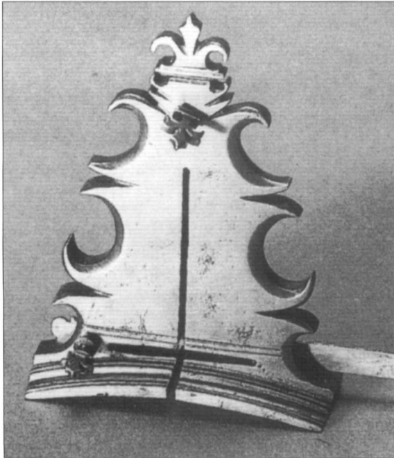
An Italian gunner's sight. The object is made of brass and is pierced with an aperture vertically. The gunner placed this sight on the breech of the gun and aimed through the aperture.
