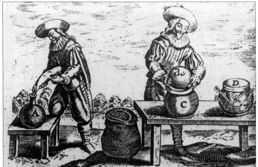
Filling mortar shells and making carcasses. This 17th-century image shows the process by which hollow cast iron projectiles were filled with gunpowder. The figure on the left is making combustible projectiles that are fitted inside an earthenware pot. (From Manneson Mallet's Les Travaux de Mars )
