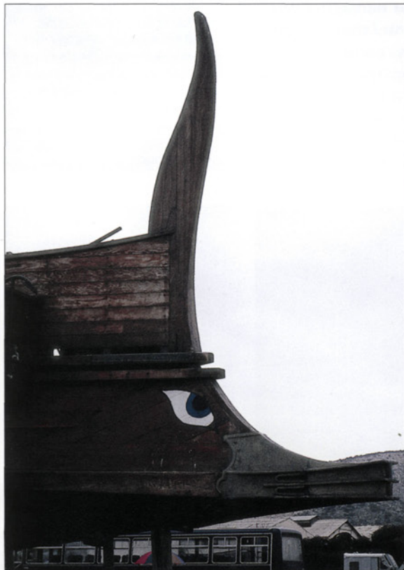
The shape of the ram was designed to cause maximum waterline damage without penetrating the hull too far and making it difficult for the attacking vessel to back off. In Olympias the bronze sheath weighs some 200kg (440lb). (Author's collection)
