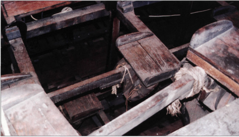
Modern rowers are able to take full advantage of the strength of their leg muscles via the use of a sliding seat. The ancient oarsman sat on a cushion atop a fixed seat. This view shows, from right to left, the seats for a thranites , zugios , thalmios and, again, a thranites . (Courtesy of William Shepherd)
